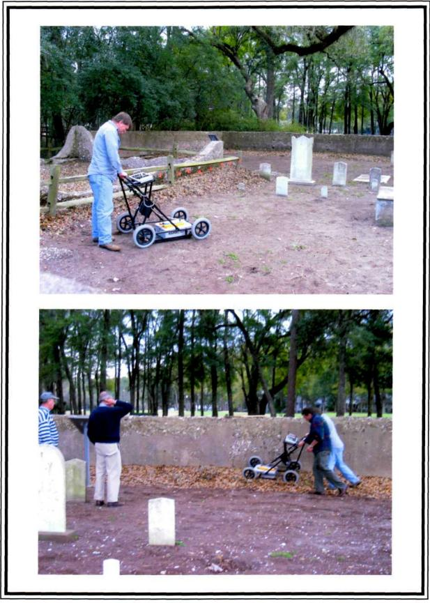
Figure 3. Views of the GPR survey of the Sams Family Cemetery at 38BU581. Top: Dr. Poplin adjusting the radar data collector prior to survey; note the pin flags defining survey transects in center of photograph. Bottom: Dr. Poplin and Mr. Greg Djouboulian pushing the GPR equipment along a survey transect.
